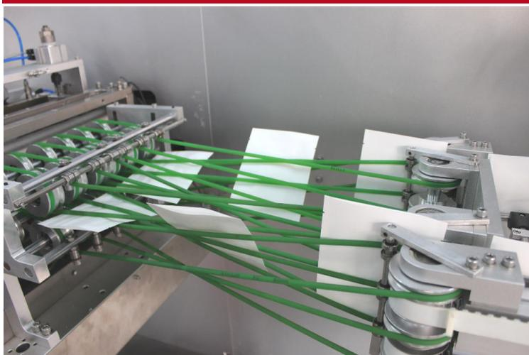
Bag transfer system (to liquid filling sealing machine)
