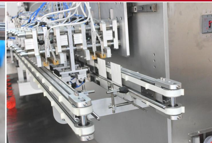
8 station sealing bars and output
