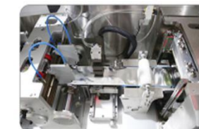
废边分切及往复易撕口部分 Both sides cutting and easy tear making
