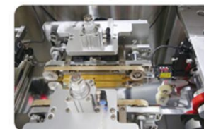
中封部件以及激光检测 Both sides sealing and laser detection
